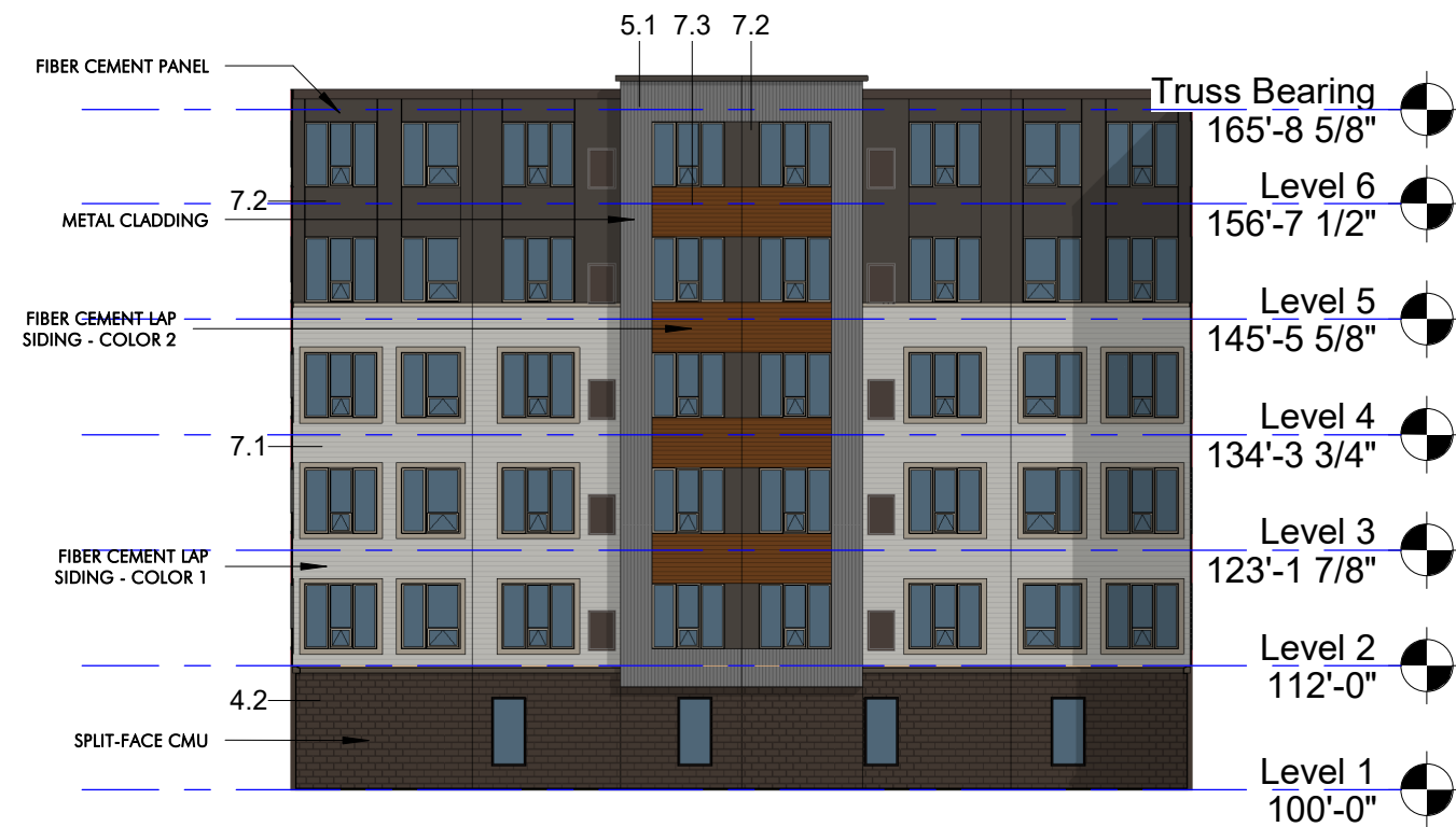
③ Elevation - Courtyard West 1" = 20'-0"
