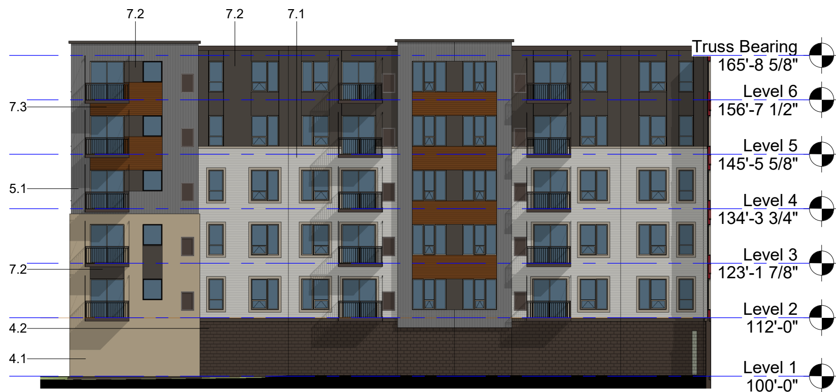
② Elevation - Courtyard North 1" = 20'-0"
