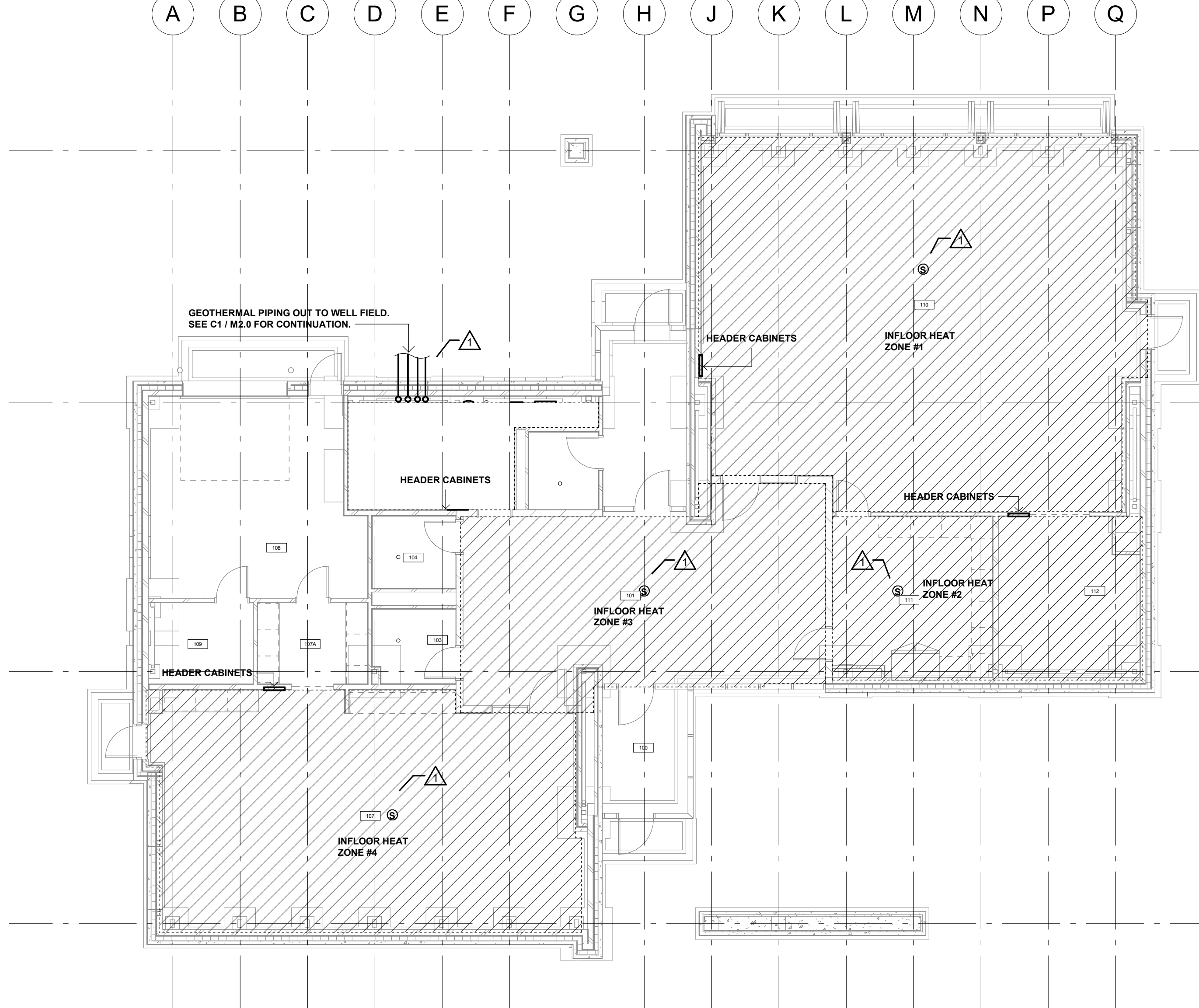
F5 HYDRONIC PIPING PLAN - INFLOOR HEATING PLAN 1/8" = 1'-0"
