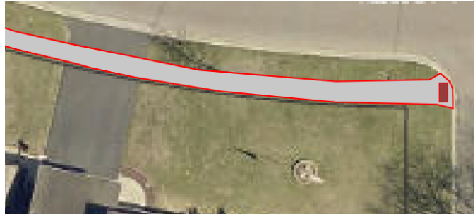
Figure 4: Sidewalk setback 1.0 foot from property line
