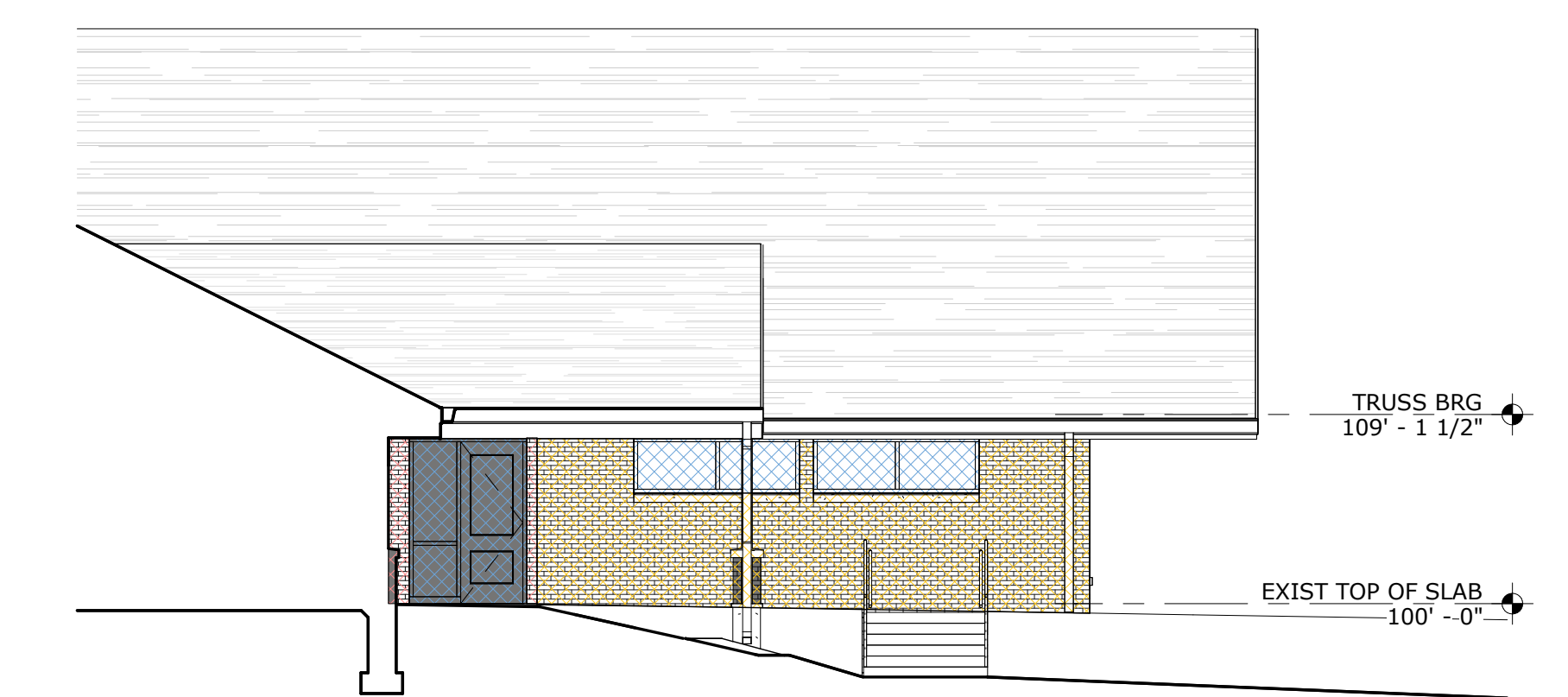
④ PARTIAL BUILDING ELEVATION WEST 1/8" = 1'-0"
